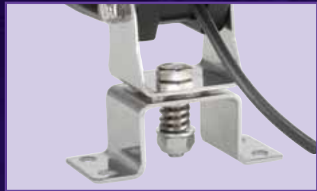
Stainless steel mounting bracket with a pressurised spring provides a sturdy yet tool-free swivel movement
