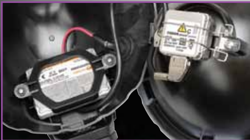
Internally mounted Gen 5 ballast and D1S globes
