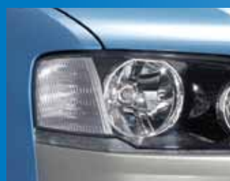
Phantom indicator globe in clear lens when not operating.
