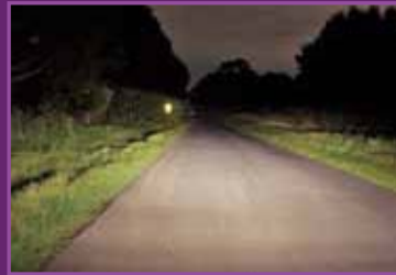
Standard 90mm headlamp using a standard 55W halogen globe
