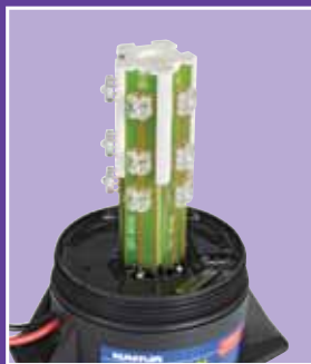
Potted electronics protects and extends circuitry life
