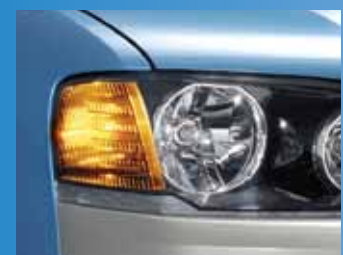
Phantom indicator globe in clear lens when flashing.
